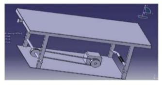
**Motor Calculations:-**Battery=24V,12.2Ah Motor=Output Power=250W Rated Voltage=24V Rated Speed=3300RPM Reduction Ratio=9.78 Speed after reduction=265RPM Torque=9N.m Wheel Diameter=70cm Cart to Carry Weight=150kg Here, Pi=Vdc×Idc=292.8 &  $Po=2\pi NT1/60$ , Eff=Po/Pi, Therefore, Tl=Eff×Pi×60/2 $\pi$ N=67.78N.m Then,  $P=2\pi NT/60$ Therefore,  $N=P\times60/2\pi\times67.78$  i.e.  $68RPM\sim5.21$ kmph. Therefore the Speed of the cart with 150kg weight is equal to 5.21kmph.
